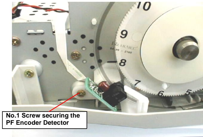
Figure 4-54. Removing the PF Encoder Sensor
